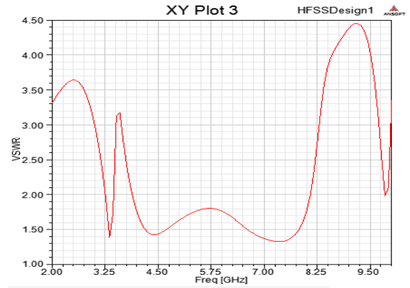
Fig. 5: Simulated VSWR parameter.
