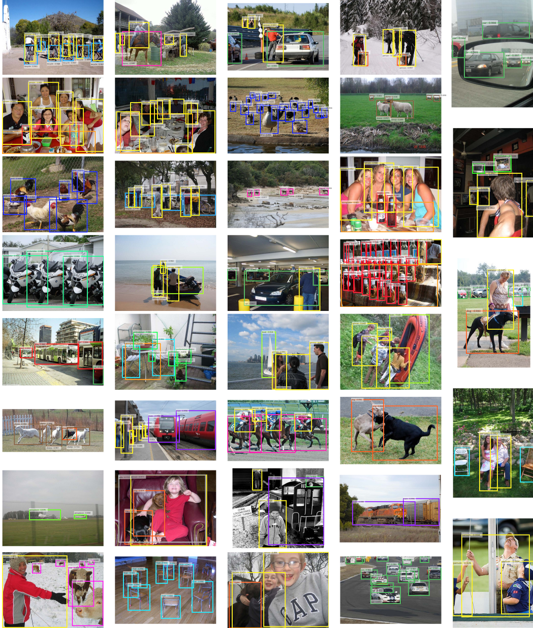
Figure 5: Curated examples of R-FCN results on the PASCAL VOC 2007 test set (83.6% mAP). The network is ResNet-101, and the training data is 07+12+COCO. A score threshold of 0.6 is used for displaying. The running time per image is 170ms on one Nvidia K40 GPU.
