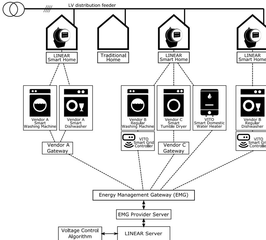
**Fig. 2.** Illustration of the technical setup of the appliances and communication channels during the pilot.
