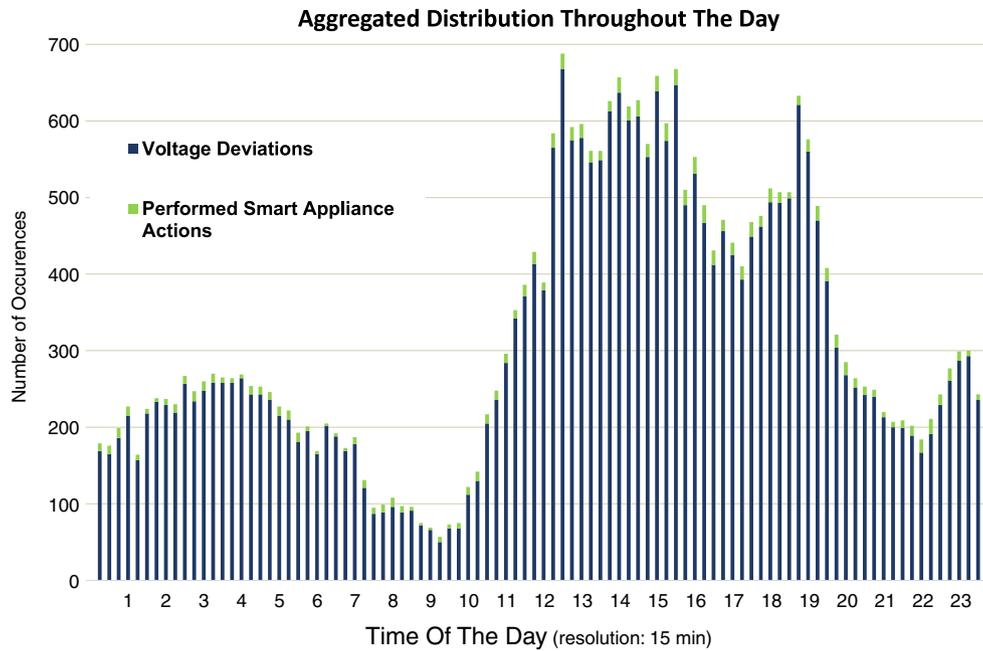
**Fig. 5.** Aggregated distribution throughout the day of the prevalence of voltage deviations and the performed smart appliance actions. The discrepancy between the amount of flexibility requested and flexibility given is due to the lack of flexible appliances at the right time on the right phase in each household.
