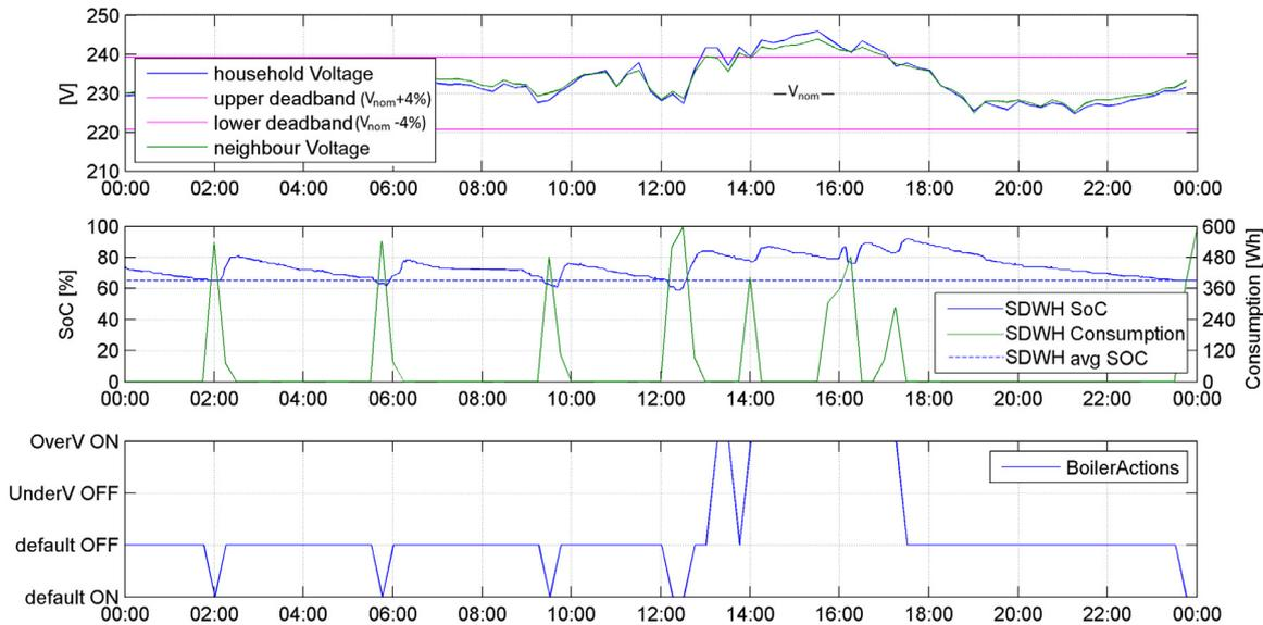
**Fig. 3.** The top chart depicts the measured voltage profile for 24 h one of the households participating in the pilot, accompanied by the voltage profile of the neighboring household. In the middle the SoC and consumption of the SDWH in this household are shown. At the bottom a visual representation of the actions that were sent to the SDWH during the day.
