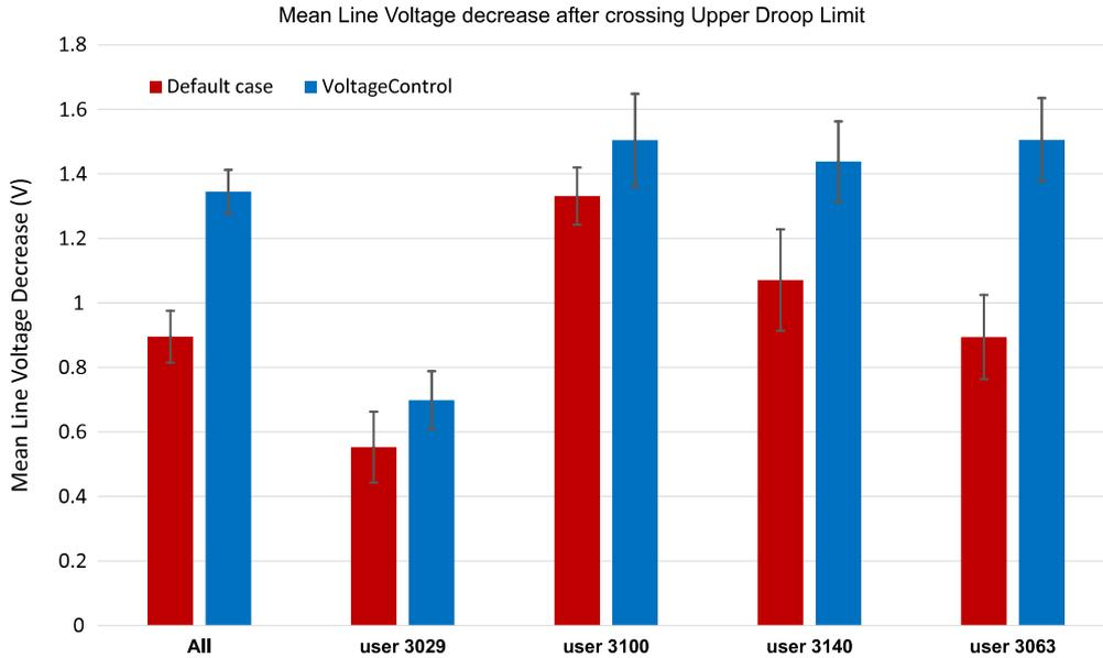
Fig. 7. Average line voltage drop for different households equipped with a SDWH for both reference case and Voltage Control case.
