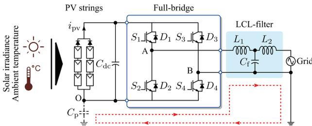
Fig. 5. Single-phase single-stage transformerless full-bridge string inverter with an LCL filter, where  $i_{pv}$  represents the PV output current and  $C_p$  is the parasitic capacitor between the PV panels (strings) and the ground. The red dashed line indicates possible leakage currents circulating through the parasitic capacitor  $C_p$ .
