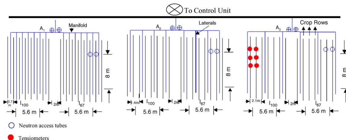
**Fig. 1 – Layout of the experimental plots, and location of tensiometers and neutron access tubes (one replication).**
