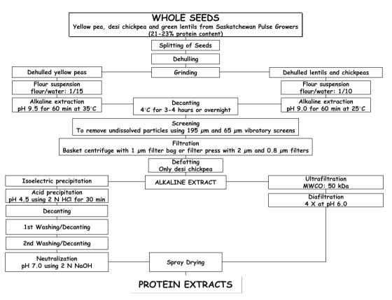
Fig. 1. Schematic of the process used for the pilot scale production of the pulse protein concentrates.
