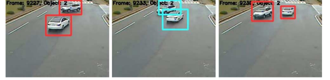
Fig. 6. The result of re-detection of occluded objects. The middle image shows the re-detected objects in the case of occlusions with the mean-shift algorithm.
