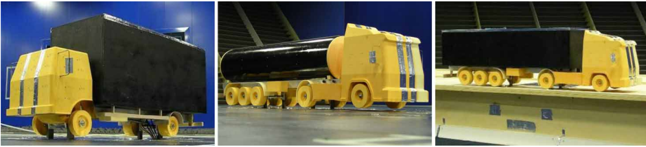
Figure 9. Scale vehicle models: van (left); tanker (centre); truck (right).
