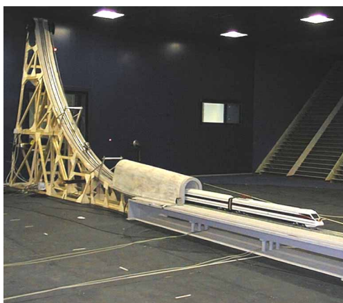
Figure 8. Moving model tests in the PoliMi wind tunnel.
