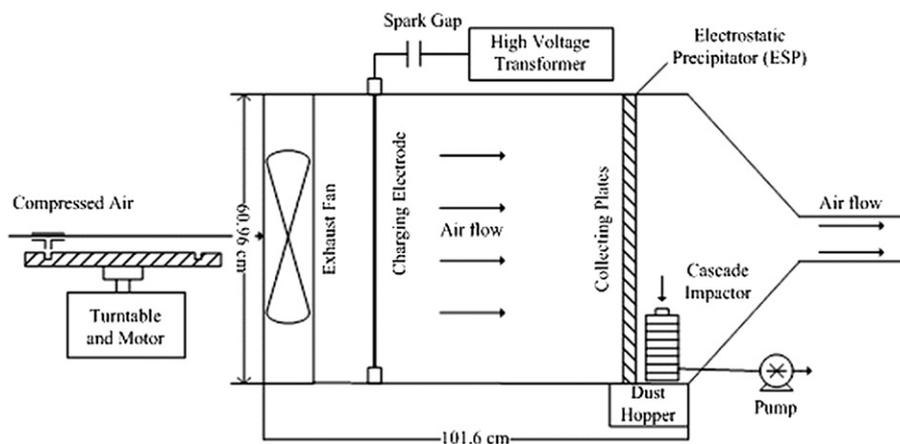
Fig. 1. Schematic drawing of the experimental setup.
