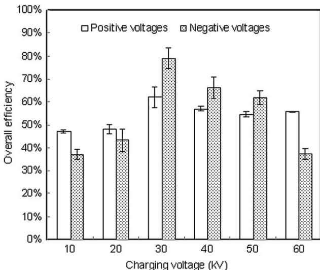
Fig. 3. Overall particle collection efficiencies under positive and negative charging voltages.
