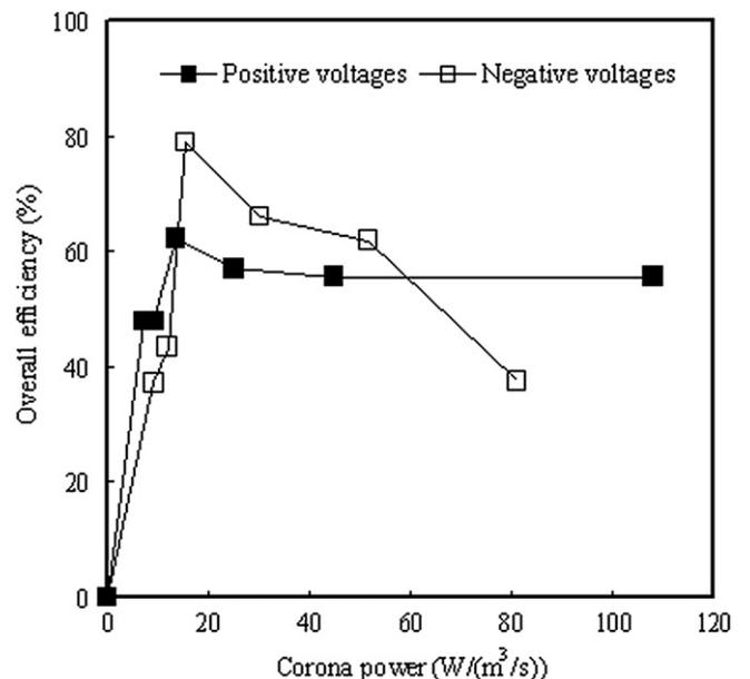
Fig. 5. Overall particle collection efficiencies based on corona power.
