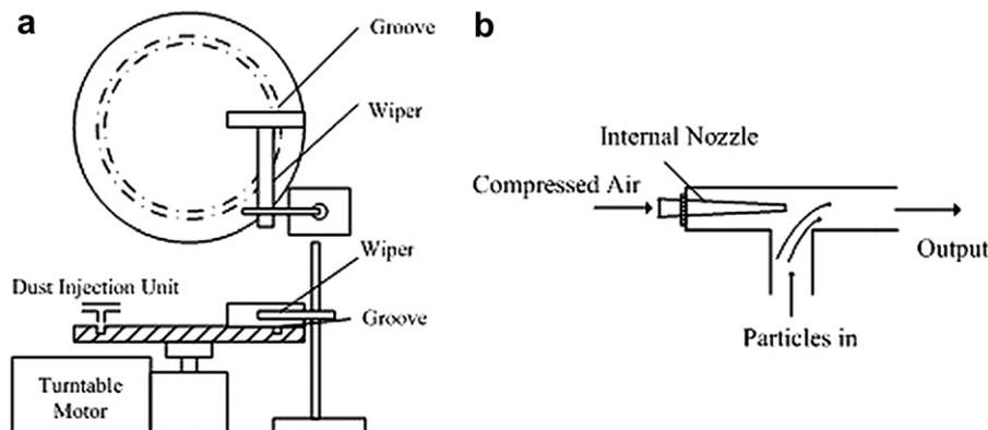
Fig. 2. (a) Schematic drawing of the turntable dust feeder. (b) Details of the dust injection unit.
