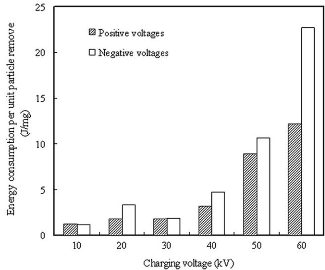
**Fig. 6.** Energy consumption per unit particle removal (unit: j/mg).
