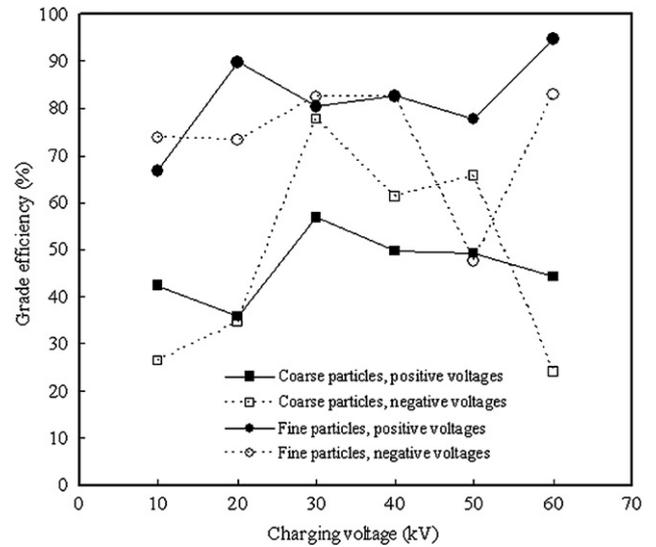
Fig. 4. Grade efficiencies of coarse and fine particles under positive and negative charging voltages (coarse particles: diameter larger than 2.1  $\mu\text{m}$ ; fine particles: diameter less than or equal to 2.1  $\mu\text{m}$ ).
