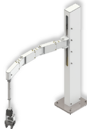
Figure 2. Scheme of a robotic manipulator with rotational and prismatic redundancy.
