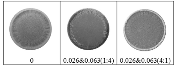
Fig. 18. Photographs of specimens in the mixtures with two sediment sizes (0.026 mm and 0.063 mm) at a concentration of 50 kg/m 3 with different ratios (1:4 and 4:1) after 240 min exposure (Cases 25 and 26).
