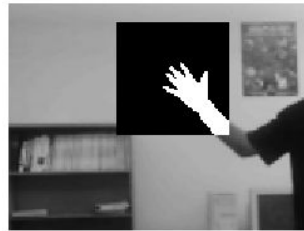
Figure 3. A ROI containing a hand. this initial ROI was found from motion detection. Then the image was differenced with the reference frame in that region and binarized, giving a segmented hand image. The size of the ROI is preset during calibration
