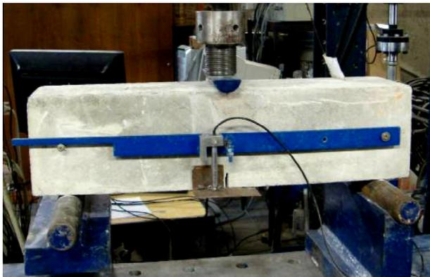
Fig. B4. Test setup of the bending test.
