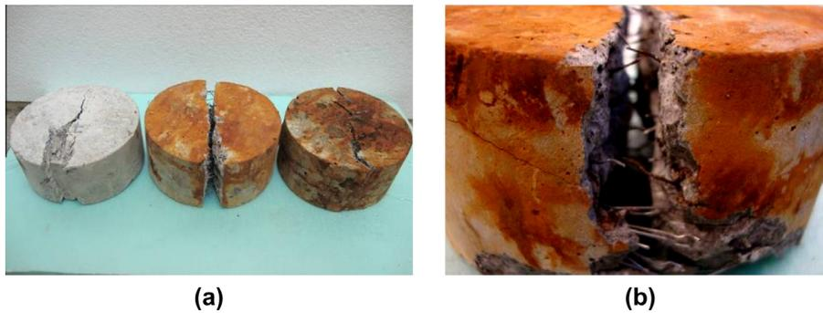
Fig. B14. SFRSCC specimens after and before chloride migration test (a) and after tensile test by diametral compression (b).
