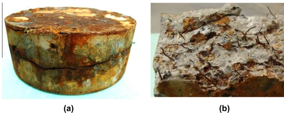
Fig. B15. Micro-cracking observed in SFRSCC specimens after chloride migration test (a) and fracture surface after diametral compression test (b).
