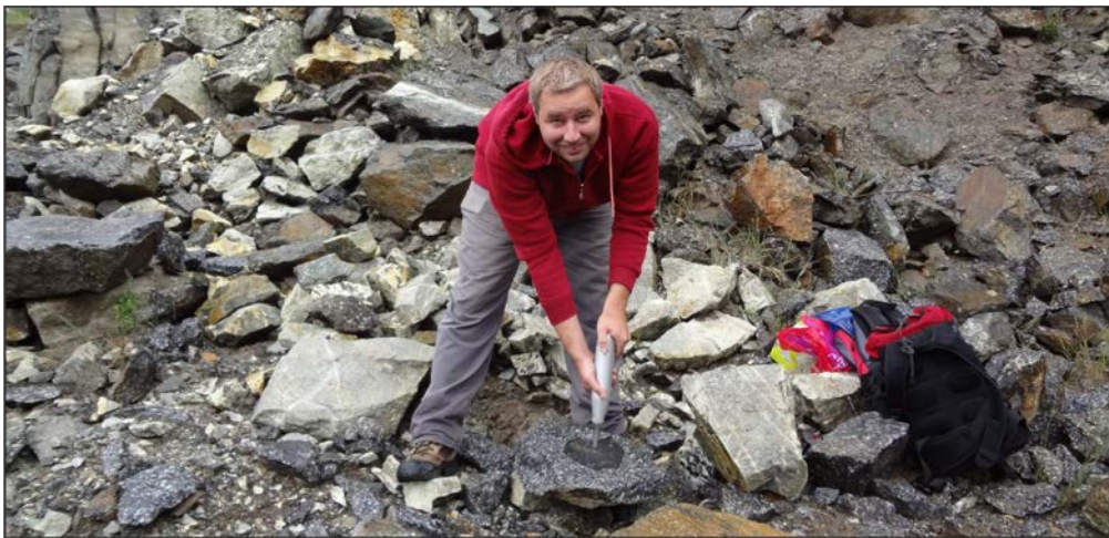
Fig. 2. Field study of the rebound hardness of multicomponent geomaterials using the N-type Schmidt hammer.
