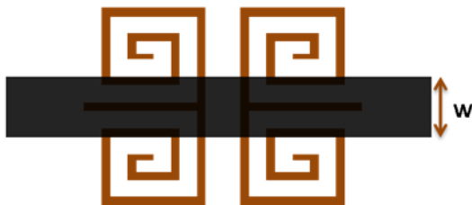
Figure 4. Transmission line with spiral structure ( w = 3 mm).
