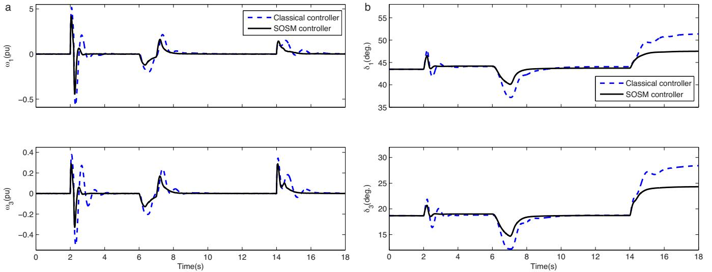
**Fig. 3.** Control response to 200 ms symmetrical three phase short-circuit fault, loss of measurable terminal voltage signal and variation of  $P_m$  (45% drop). (a) Relative rotor speed. (b) Power angle.
