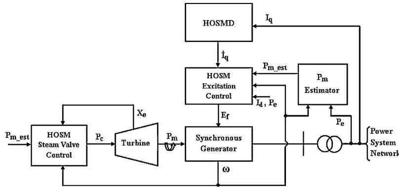
Fig. 1. Block diagram of proposed control scheme.
