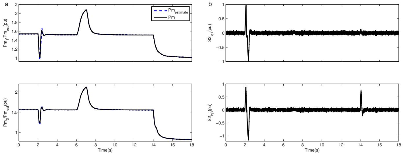
**Fig. 6.** Control response to 200 ms symmetrical three phase short-circuit fault, loss of measurable terminal voltage signal and variation of  $P_m$  (45% drop). (a) Mechanical power input and its estimate. (b) HOSMD estimation errors of the time derivative of  $I_q$ .
