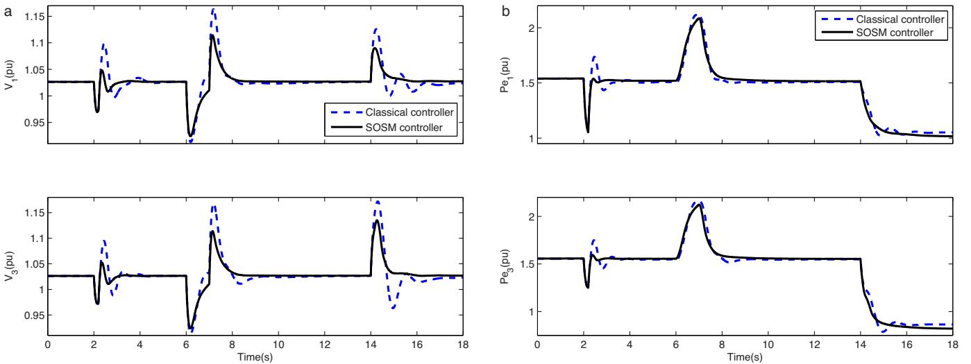
**Fig. 4.** Control response to 200 ms symmetrical three phase short-circuit fault, loss of measurable terminal voltage signal and variation of  $P_m$  (45% drop). (a) Terminal voltage. (b) Active electrical power.
