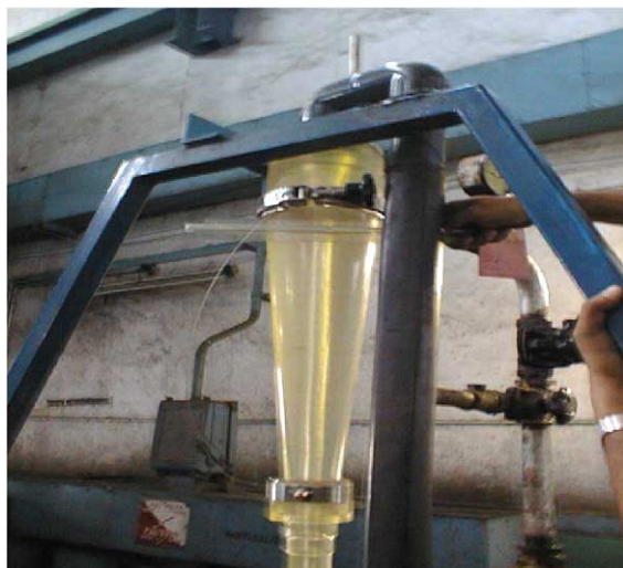
Fig. 2. Laboratory hydrocyclone (diameter: 101 mm, vortex finder 35 mm and spigot: 10 mm).
