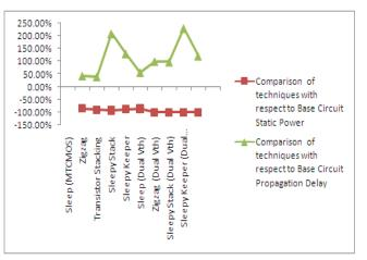
Fig. 16. Simulation Results of 1-bit adder at 70nm
