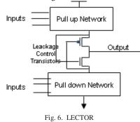
The gate of PMOS LCT is connected to the drain of pull down network while the gate of NMOS LCT is connected to the drain of the pull up network. With this wiring, with any input combination during standby mode one of the two LCTs is always near its cut-off region. This increases the resistance of the path from supply voltage to ground thus reducing the leakage power.
