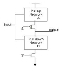
Fig. 4. Transistor Gating Technique
