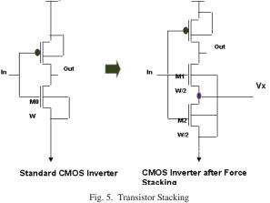
Because of all the above points, the leakage reduction factor is changed reducing the leakage current.
