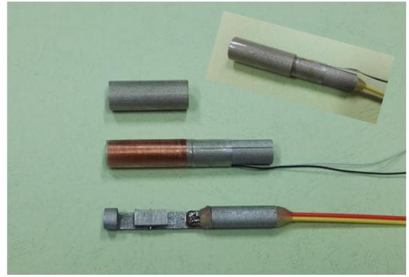
**Fig. 2.** (Color online) Structure of the sensing head consisting of the MPLC, the modulation coil, and some auxiliary mechanisms.
