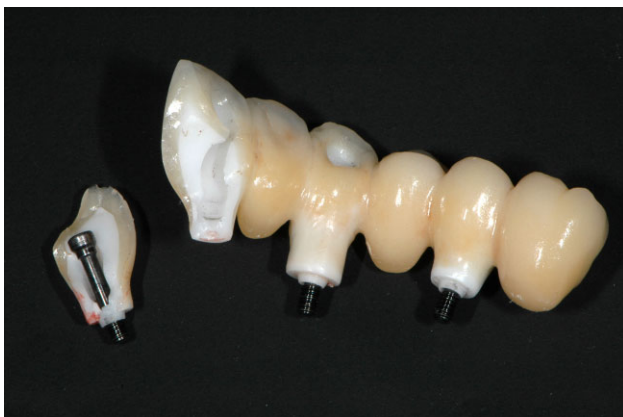
Figure 4 Six-unit FPD, fracture of framework.
