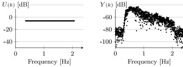
**Fig. 5.** Spectra (•) (in dB) for the LPV IO model (38), over the entire measurement record. (left) The input is a random phase multisine (1), which has a flat amplitude spectrum. (right) Corresponding output spectrum, for a scheduling signal  $\in [-1, 1]$  with 20 harmonic frequencies.
