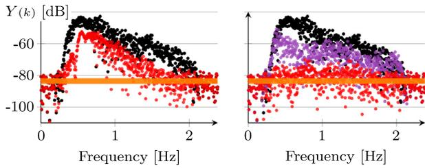
**Fig. 8.** (left) True output spectrum ( $\bullet$ ) of the initial static approximation, given the time-varying state space realization of (38). The error ( $\bullet$ ) lies far above the noise standard deviation ( $\text{—}$ ). (right) Optimized polynomial state space model. The error ( $\bullet$ ) of the indirect method is comparable with the noise level ( $\text{—}$ ). The error of the optimized BLTI model ( $\bullet$ ) cannot reach the noise floor.
