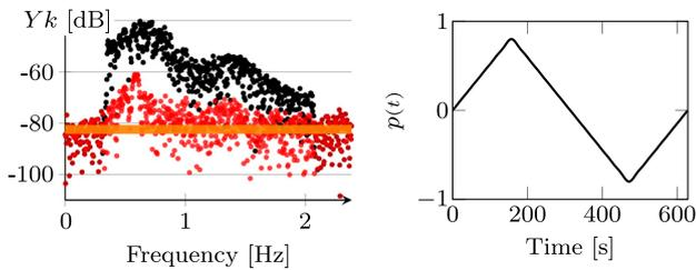
**Fig. 10.** (left) True output spectrum ( $\bullet$ ) and model error ( $\bullet$ ) of the estimated LPV state space model, for the triangular validation scheduling trajectory (right). The error increases a little w.r.t. Fig. 8, but the order of magnitude is still similar to the noise standard deviation ( $\text{—}$ ).
