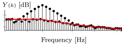
**Fig. 3.** Output spectrum  $Y(k)$  of a periodic parameter-varying system for a single sine excitation. Energy appears only at the harmonic frequencies. If multiple periods are measured, a non-parametric noise model (–) can be estimated.
