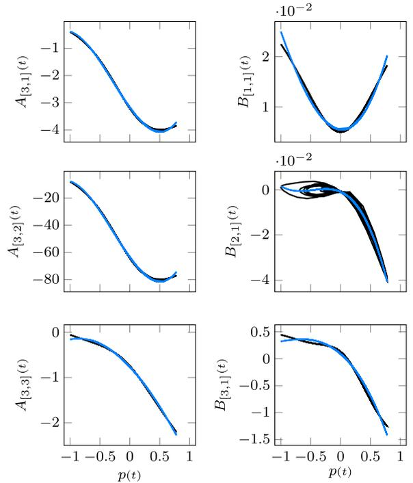
**Fig. 7.** Realized time-varying state space coefficients (–)  $A_{[i,j]}(t)$  and  $B_{[i,j]}(t)$ , plotted against the scheduling signal  $p(t)$ . The static parameter-varying coefficients, obtained via least squares regression with a polynomial basis functions  $\phi_i(p(t)) = p(t)^i$  are shown on top (–).
