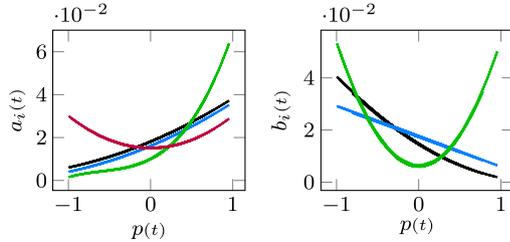
**Fig. 6.** Normalized time-varying coefficients  $a_i(t)$  and  $b_i(t)$ , with respect to the scheduling signal  $p(t)$ . From these plots, we can deduce the polynomial order  $N_p$ , and verify that the differential equation can be modeled with static coefficients.
