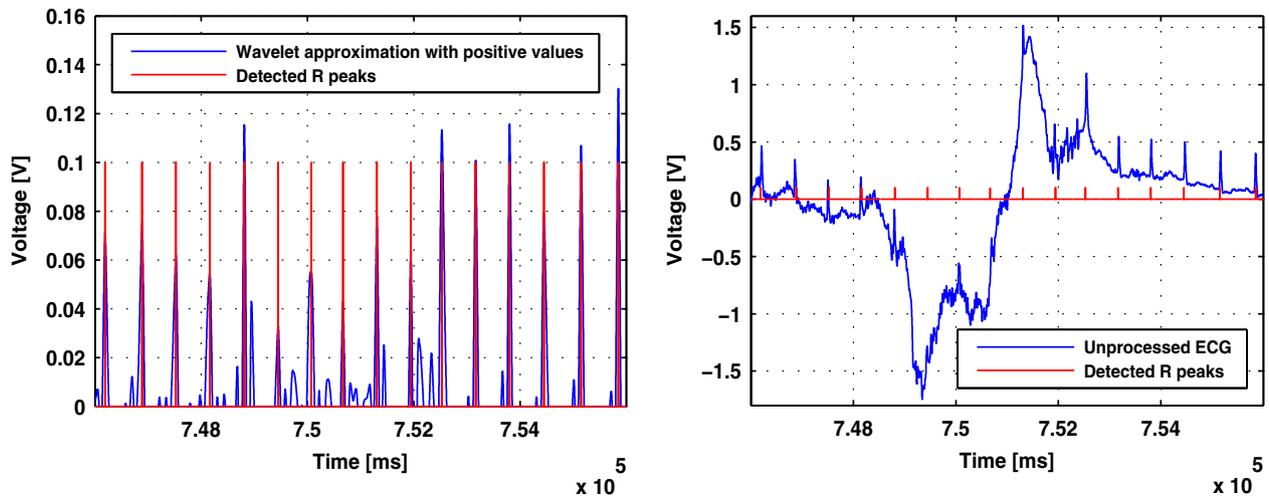
Fig. 6. R peaks detected in the wavelet approximation and in the original ECG.
