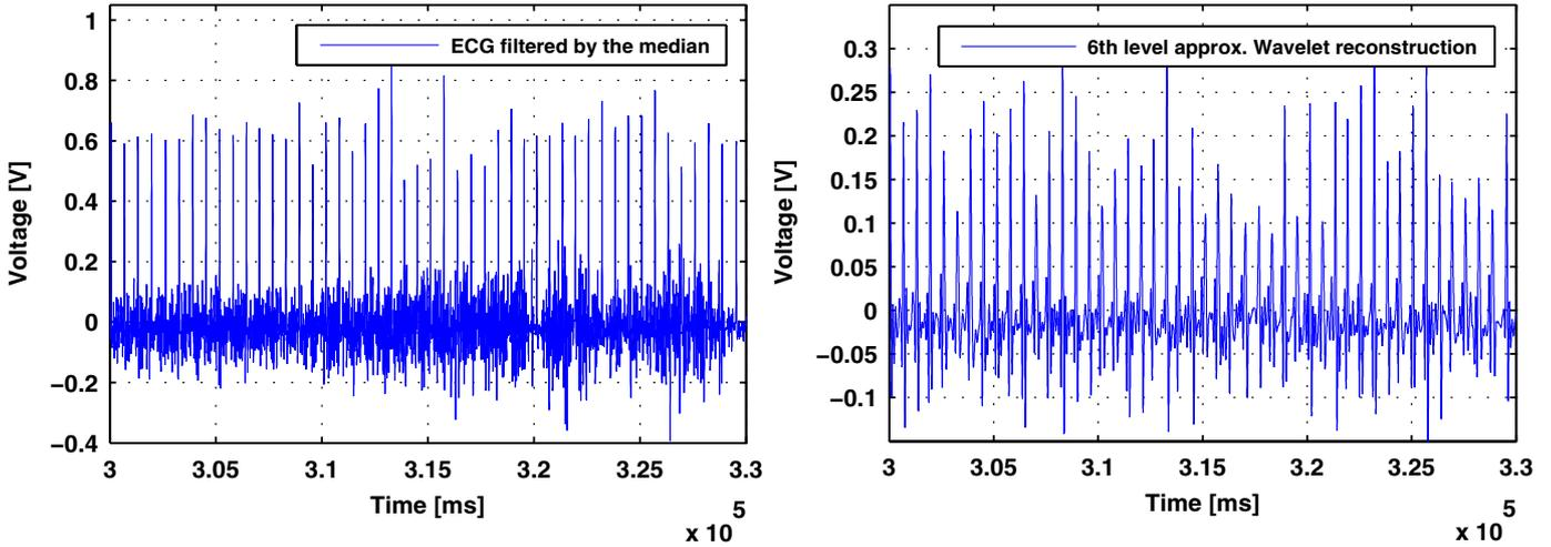
Fig. 5. Noise filtering by the 6th wavelet approximation.
