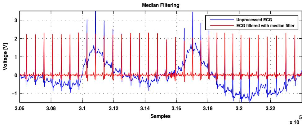
Fig. 3. Offset artifacts removed from the original signal by applying the median filter.
