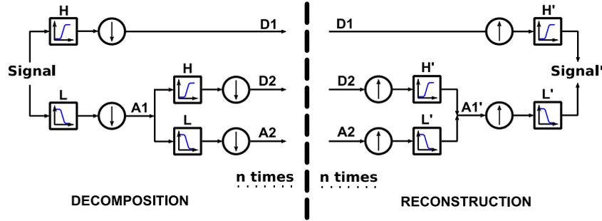
Fig. 4. Wavelet decomposition and reconstruction scheme.
