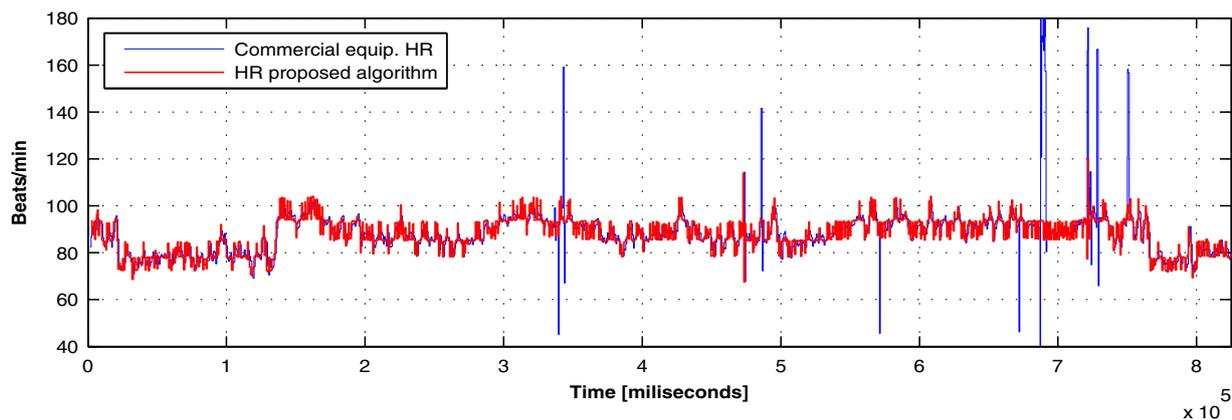
Fig. 7. The calculated HR and the obtained from the commercial equipment.
