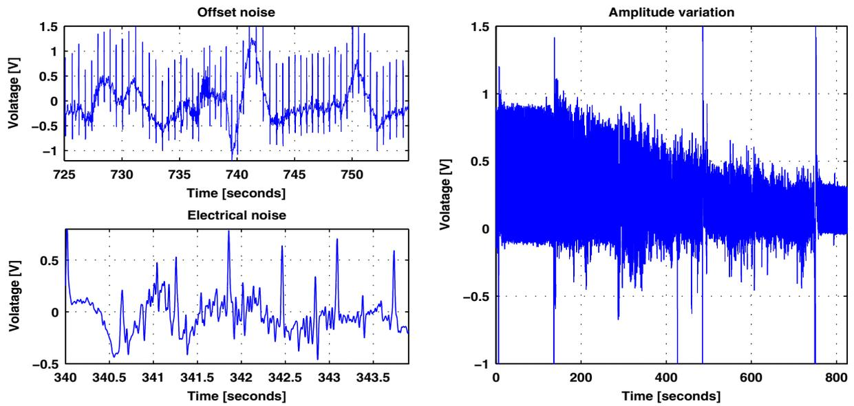
Fig. 2. Different noises and artifacts produced in the ECG signal.
