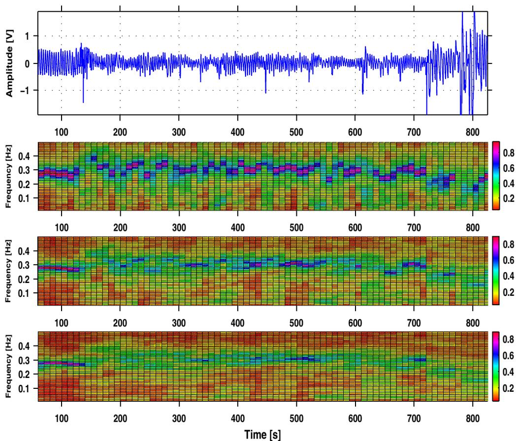
Fig. 9. Correlation between pure sine waves and the RESP signal by different windows.
