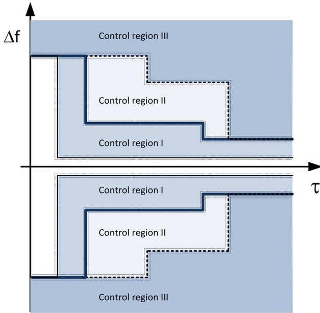
Fig. 3. Aggregated load controller  $\Delta f$ - $\tau$  characteristic. Different load groups.
