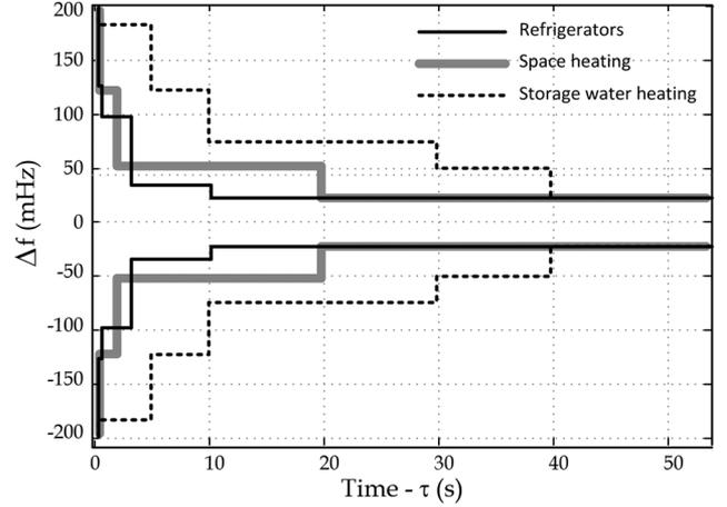
Fig. 6. Average  $\Delta f$ - $\tau$  switching characteristics used in simulations.
