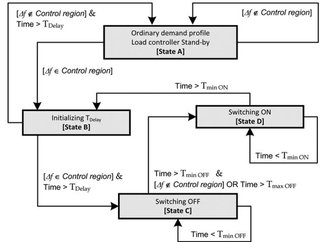
Fig. 4. Finite state machine representation of the load controller. Underfrequency.
