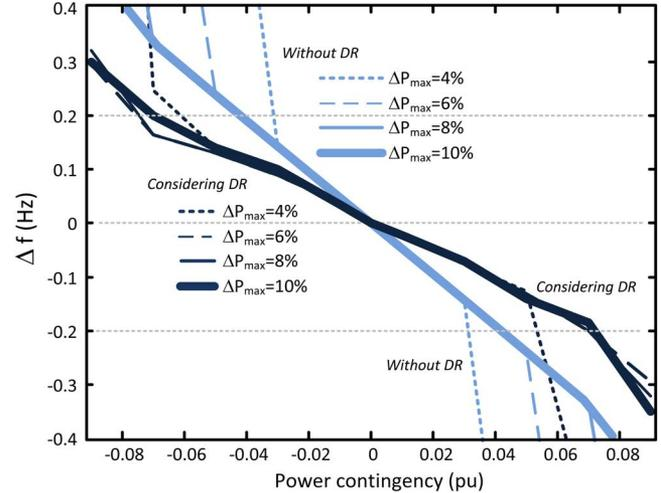
Fig. 10.  $\Delta f$  average simulated values with different amounts of primary frequency response available from the generation.
