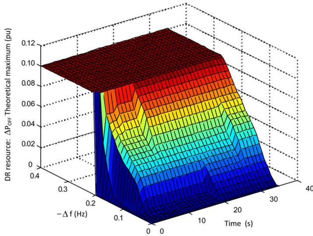
Fig. 7. Simulated DR aggregated behavior. Underfrequency.
