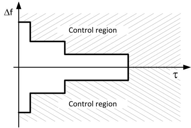
Fig. 2. Individual load controller  $\Delta f$ -time characteristic.
