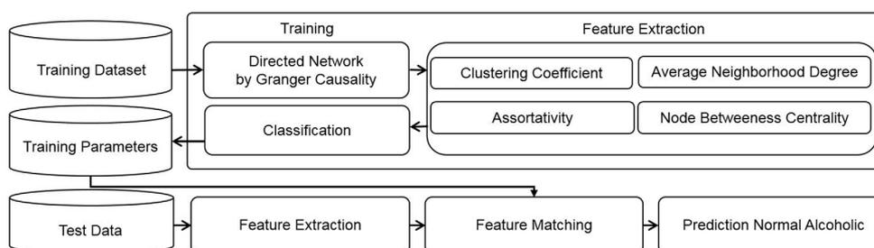
**Figure 1.** Block diagram of the proposed system for distinguishing between normal subjects and alcoholics. This data mining framework uses network properties, which are used to express the state of brains with the following parameters: clustering coefficient, assortativity, average neighborhood degree, and node between-ness centrality.
