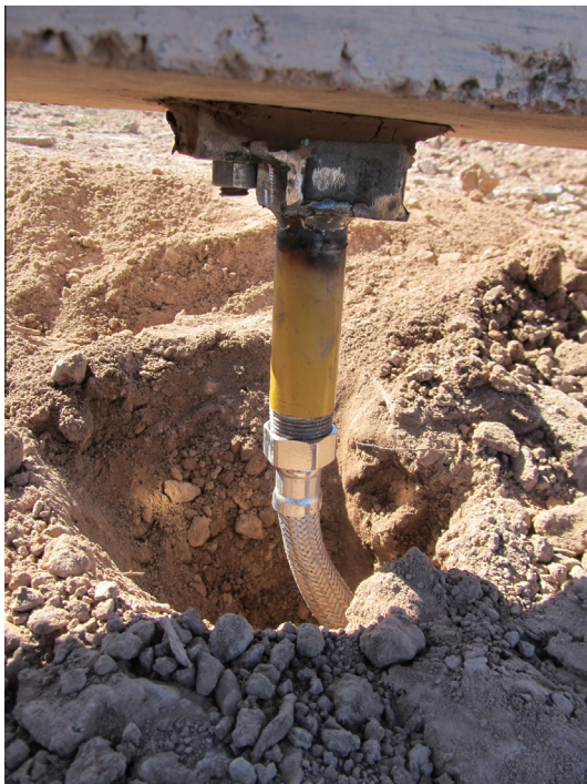
Fig. 6. View of the installed accelerometer.
