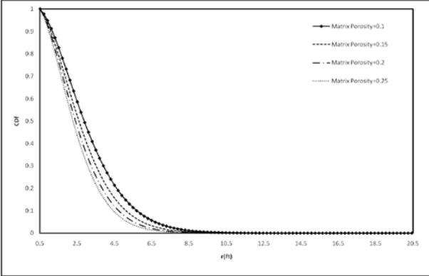
Fig. 7: Effect of Matrix Porosity on Filtrate Transport
