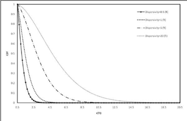
Fig. 9: Effect of Dispersivity on Filtrate Transport
