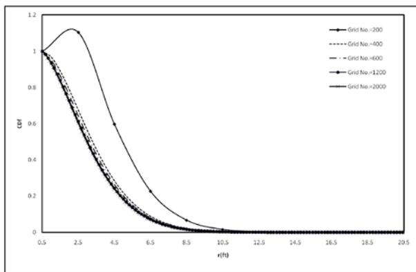
Fig. 3: Effect of Grid Number in Radial Direction on Filtrate Transport
