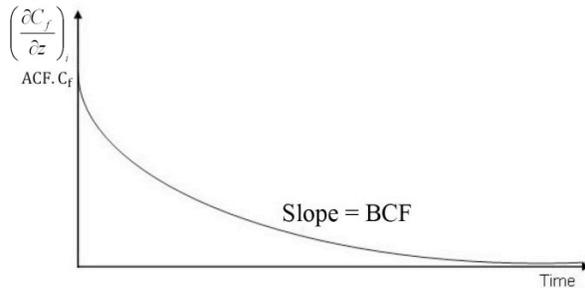
Fig. 2: Concentration Gradient at the Interface versus Time
