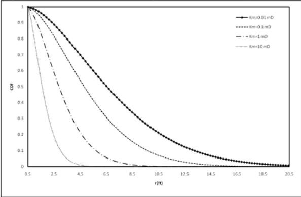
Fig. 8: Effect of Matrix Permeability on Filtrate Transport
