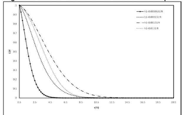
Fig. 6: Effect of Fracture Opening Size on Filtrate Transport
