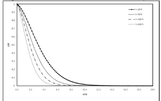
Fig. 5: Effect of Reservoir Thickness on Filtrate Transport
