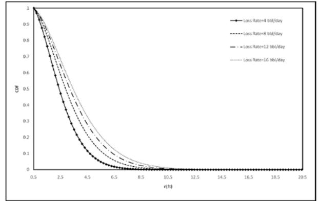
Fig. 4: Effect of Wellbore Loss Rate on Filtrate Transport
