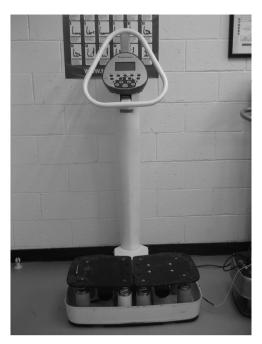
Fig. 1. Dual-plate whole-body vibration machine.
