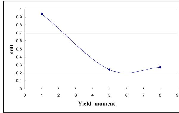
**Figure 9.** The maximum displacement of the frame versus yield moment
