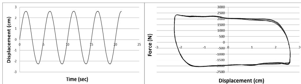
**Figure 5.** The applied displacement loading with displacement amplitude of 2.5 cm and its hysteresis load deflection curve of the device
