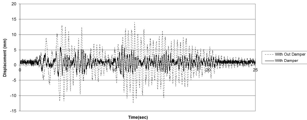
**Figure 10.** Time-displacement curve of the SDOF frame with the damper under Tabas earthquake excitation
