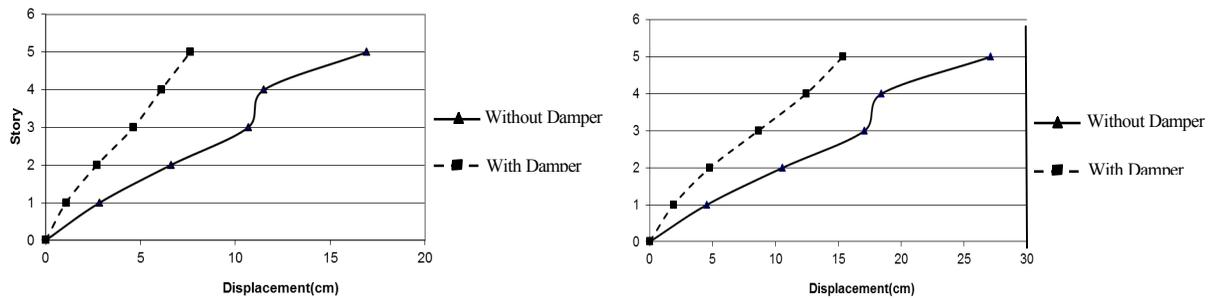
**Figure 13.** Displacements of the five story structure under Tabas scaled excitation 0.35g ( left ) , 0.5g ( right )
