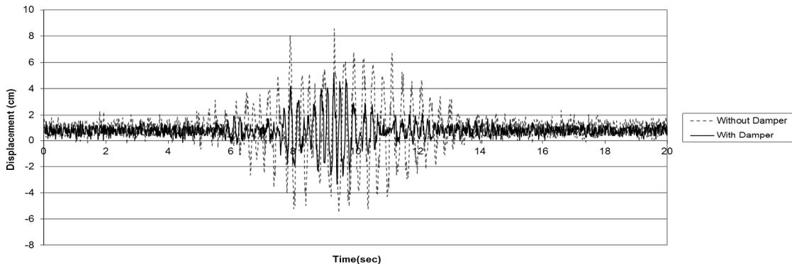
**Figure 11.** Time-displacement curve of the SDOF frame with the damper under Kobe earthquake excitation
