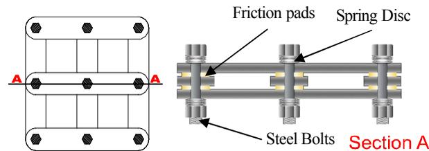
Figure 1. Friction damper and A-A cross section
