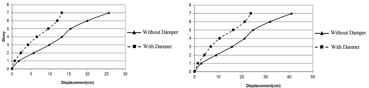
**Figure 14.** Displacements of the seven story structure under Tabas scaled excitation 0.35g ( left ) , 0.5g ( right )
