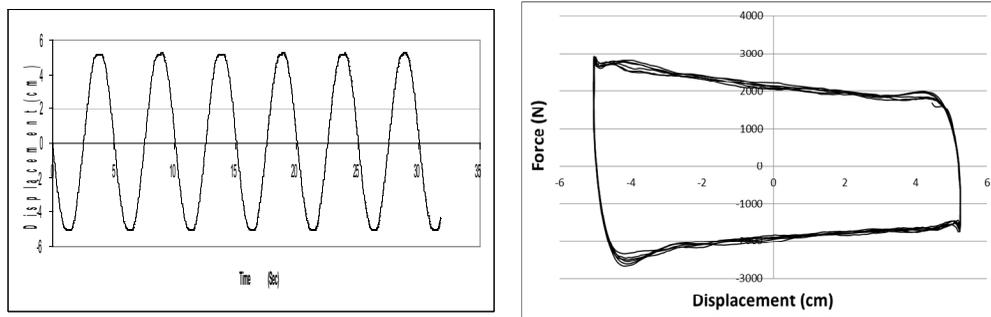
**Figure 7.** The applied displacement loading with displacement amplitude of 5 cm and its hysteresis load deflection curve of the device
