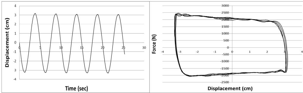
**Figure 6.** The applied displacement loading with displacement amplitude of 3 cm and its hysteresis load deflection curve of the device
