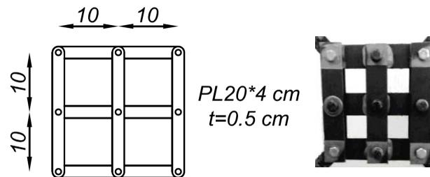
**Figure 4.** Dimensions of the prototype device
