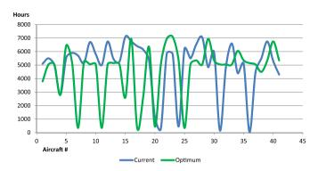
**Fig. 3.** Total number of hours  $(H_j)$  on each aircraft under current and optimum strategies.
