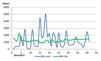
**Fig. 5.** Total number of hours  $(x_j)$  added to each aircraft under optimum solutions for minimum cost and minimum number of maintenance strategies.
