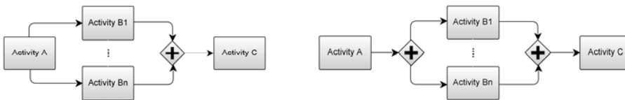
Figure 3 - BPMN patterns for Parallel process blocks
