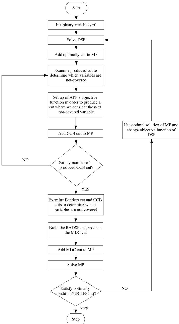
**Fig. 2** The flowchart of combination CCB and MDC methods
