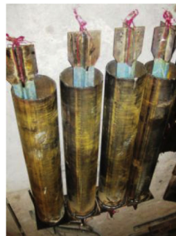
Fig. 2. Fabrication of BRB specimens. (a) The inner cores of BRBs, (b) The surfaces of inner cores were wrapped with plastic film, (c) The inner cores were located in steel tubes, (d) The concrete was casted into steel tubes.
