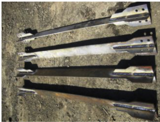
Fig. 2. Fabrication of BRB specimens. (a) The inner cores of BRBs, (b) The surfaces of inner cores were wrapped with plastic film, (c) The inner cores were located in steel tubes, (d) The concrete was casted into steel tubes.
