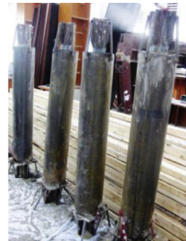
Fig. 2. Fabrication of BRB specimens. (a) The inner cores of BRBs, (b) The surfaces of inner cores were wrapped with plastic film, (c) The inner cores were located in steel tubes, (d) The concrete was casted into steel tubes.
