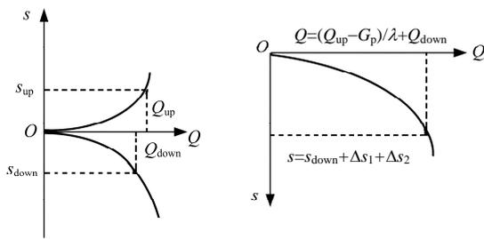
(a) O-cell load-settlement curve. (b) Equivalent load-settlement curve.
