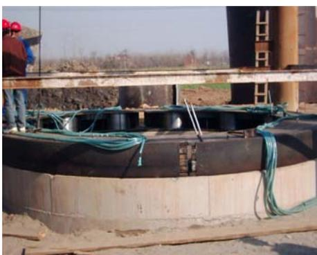
**Fig. 5** Load cell for caisson testing.
