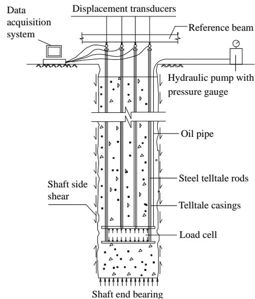
Fig. 1 Sketch of bi-directional static loading test.
