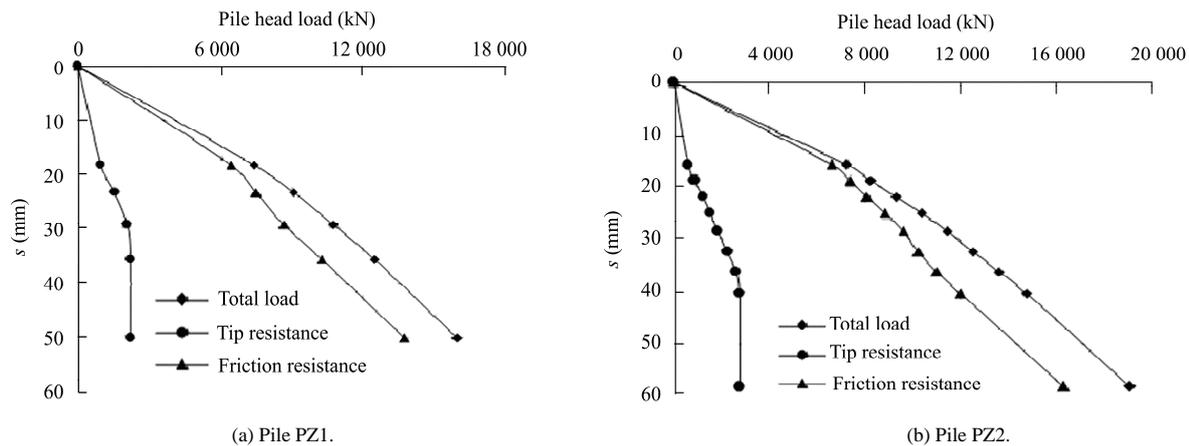
Fig. 8 The equivalent conversion curves of pipe piles PZ1 and PZ2.
