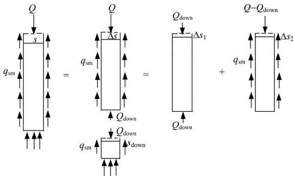
Fig. 2 Sketch of the pile head settlement calculation.
