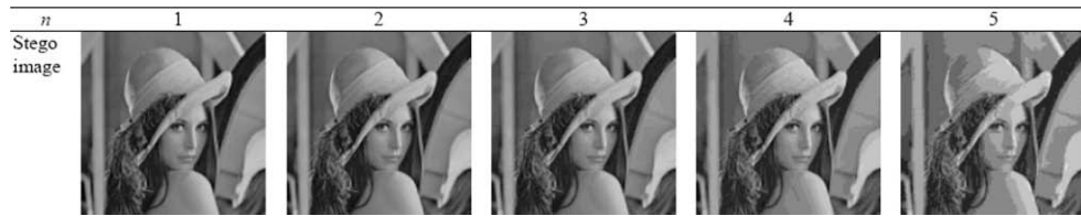
Fig. 3. The quality of the stego image when the number of LSBs changes from 1 to 5.
