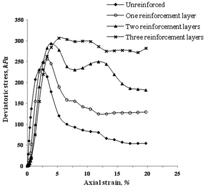
Fig. 5. Stress-Strain curves for unreinforced and reinforced clay of type II with several layers of first type geotextile for the moisture content 22% and the relative compaction of 90%.
