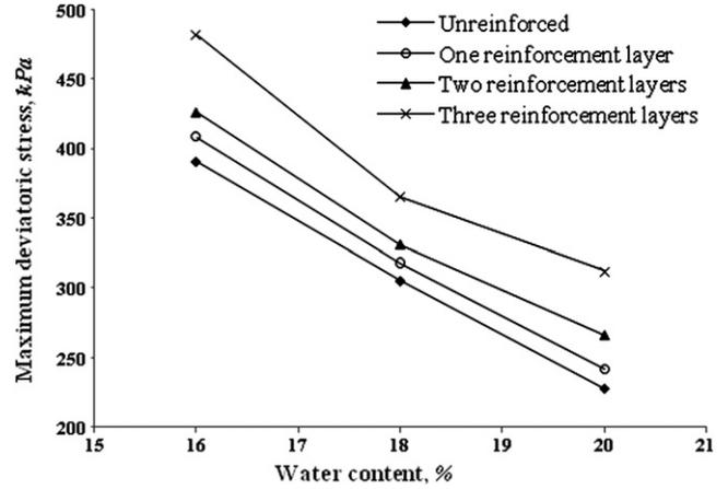
Fig. 7. The variations of unconfined peak strength based on moisture content for type I clay with relative compaction of 95% with different numbers of geotextile layers of the first type.
