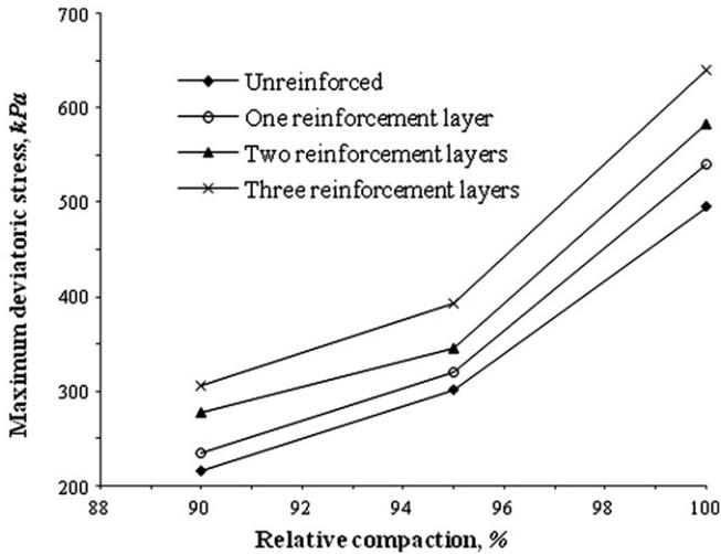
Fig. 9. The variations of peak strength based on relative compaction for type II clay with moisture content of 20% for different numbers of geotextile layers of the first type.
