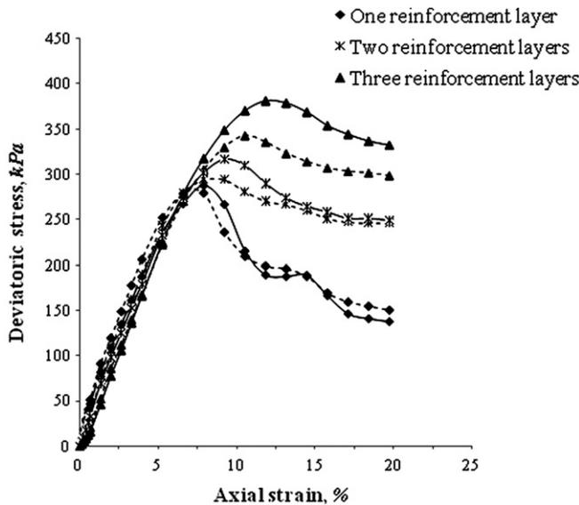
Fig. 6. Stress-Strain curves for type I clay with relative compaction of 100% and moisture content of 20%: first type geotextile (solid line) – second type geotextile (dashed line).
