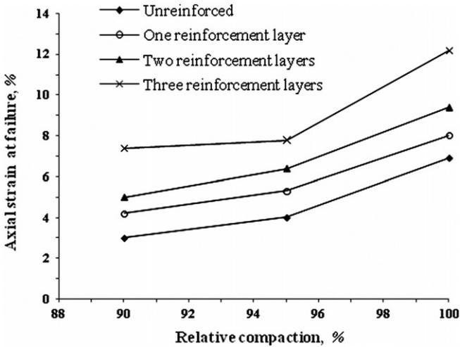
Fig. 10. The variations of axial strain at failure based on relative compaction for type I clay with moisture content of 20% with different numbers of geotextile layers of the first type.
