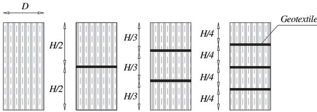
Fig. 1. The arrangement of geotextile in different samples.
