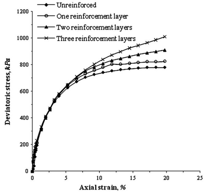
Fig. 11. Stress–Strain curves for unreinforced and reinforced clay of type I, for the relative compaction of 95% and the confining pressure 600 kPa.
