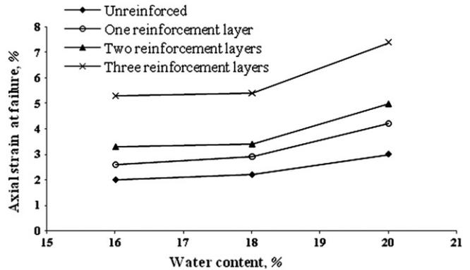
Fig. 8. The variations of axial strain at failure based on moisture content for type I clay with relative compaction of 90% for different numbers of geotextile layers of the first type.
