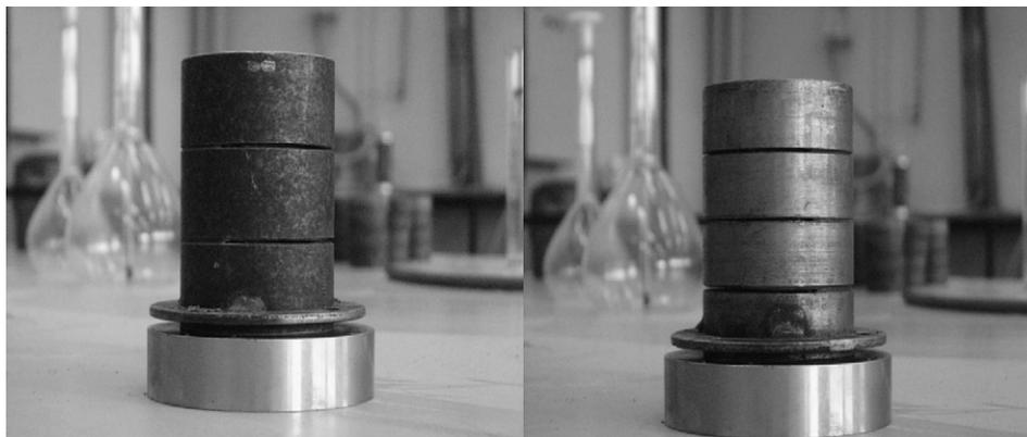
**Fig. 4.** View of the molds used for preparing the reinforced samples.
