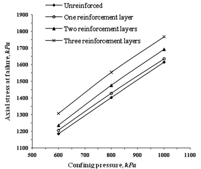
Fig. 12. Failure envelopes for unreinforced and reinforced clay of type I for different numbers of geotextiles of first type for the relative compaction of 90%.
