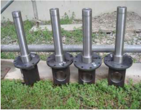
Figure 4. Anchors for ACM brace
