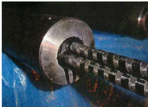
Figure 21. Steel sleeve with three CFRP rods
