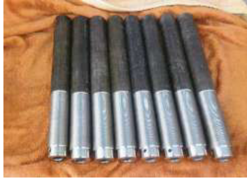
Figure 12. Steel sleeves for ACM brace
