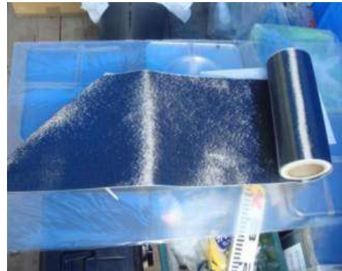
Figure 7. CFRP sheet for ACM brace
