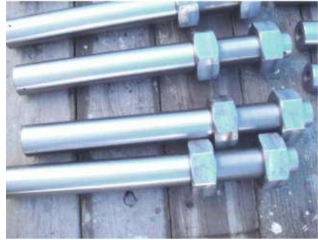
Figure 5. Steel sleeves for ACM brace
