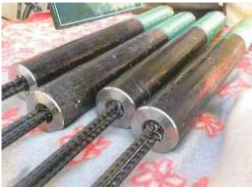
Figure 24. Steel sleeves after Epoxy resin injection work
