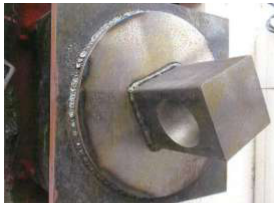
Figure 19. Steel anchor after welding work
