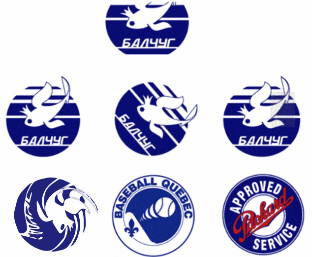
Fig. 2. Example of image retrieval results when the database contains the original and damaged versions of logos: A query image (top) and six retrieved logos ordered according to their similarity to the query logo.
