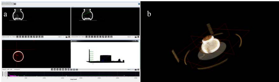
Fig. 4. (a) Example of 3D projection images in the 3 spatial directions, completed with 2D plot of axial slices; (b) 3D opacity rendering
