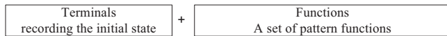
Fig. 4. Representation of a design by concatenating the terminals part and the functions part.
