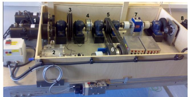
1 – DC motor (wind turbine simulator) 5 – Belt transmission system
