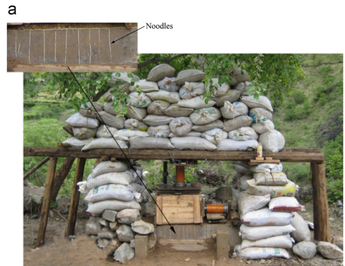
Fig. 10. Shear box used for the direct shear tests: (a) the picture of the upper shear box (60 cm × 60 cm × 40 cm) and (b) the cross section of the upper shear box (unit: cm).
