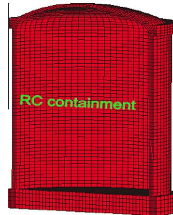
Fig. 6. The Lagrangian meshes.
