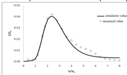
Fig 1 BTC measured value and simulation value of Ammonia - N in 15cm saturate sandy loam
