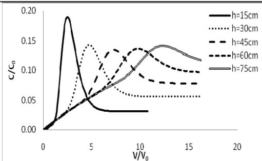
Fig 5 transportation simulation of 5mg/L Ammonia - N in different soil density
