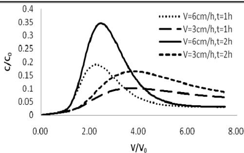
Fig 4 transportation simulation of 5mg/L Ammonia - N in saturated sandy loam before and after soil blockage
