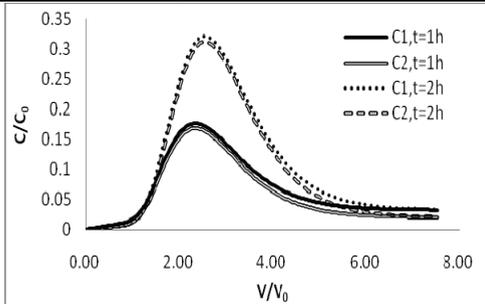
Fig 2 transportation simulation of different concentrations of Ammonia - N in saturated sandy loam
