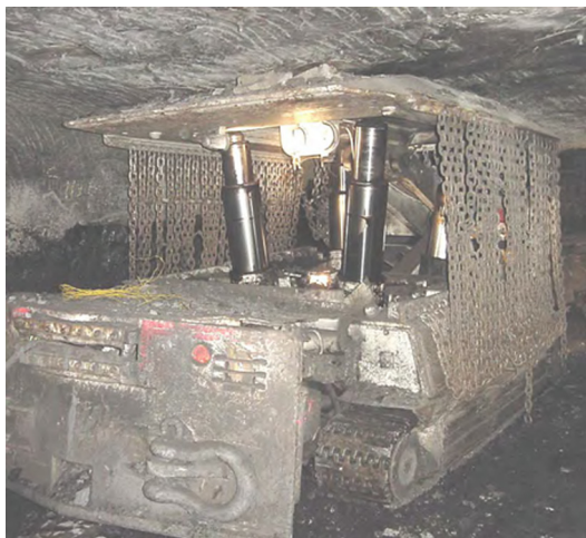
Fig. 7. A mobile roof support.
