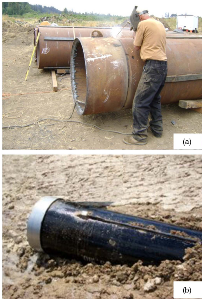
Fig. 3. Photos of typical cutting shoe options: (a) T1 steel, external cutting shoe with interior bevel (Oregon State Univ. Pipe Ramming Project); (b) steel band cutting shoe with lubrication conduit and port shown in the foreground (Najafi et al. 2005, with permission from the Missouri Dept. of Transportation)
