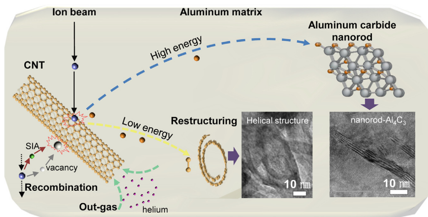
Figure 1 Schematic illustration of shape changes on CNT, recombination, and helium out-gas. Under ion irradiation, the disintegration of CNT and formation of aluminum carbide (blue arrow) from high energy ion and restructuring to helical CNT structure (yellow arrow) from low energy ion are indicated. (For interpretation of the references to color in this figure legend, the reader is referred to the web version of this article.)
