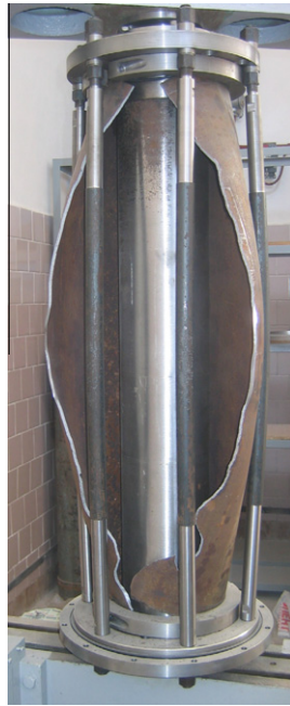
Fig. 5. Specimen after fracture.
