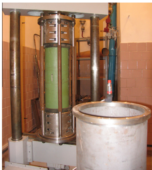
Fig. 4. Experimental device for burst test under gas pressure.
