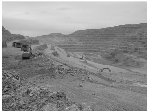
Fig. 7. An example of waiting time for loading trucks.
