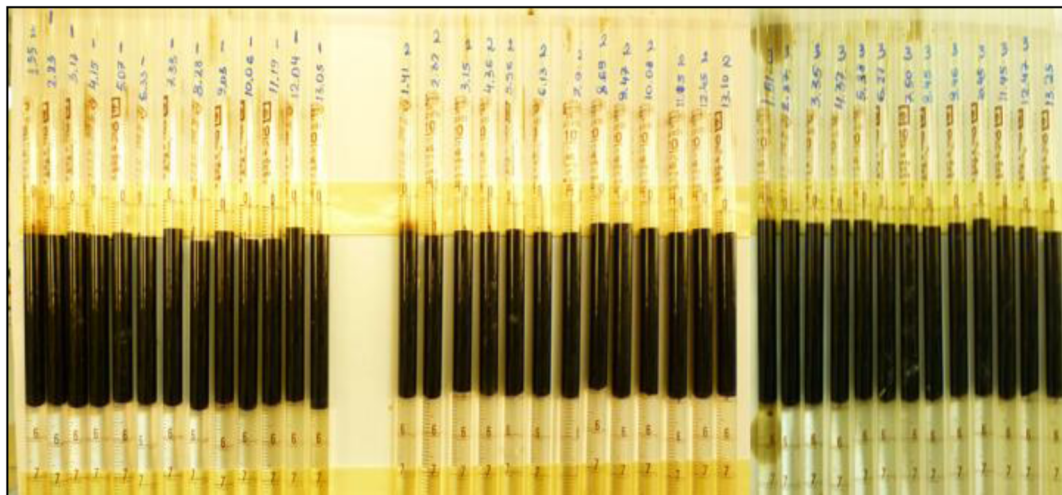
Figure 3—Microemulsion phase behavior study between crude oil and brines at different pH values (Day 7)
