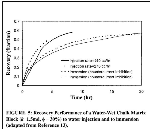
FIGURE 5: Recovery Performance of a Water-Wet Chalk Matrix Block ( $k=1.5 \text{ md}$ ,  $\phi = 30\%$ ) to water injection and to immersion (adapted from Reference 13).
