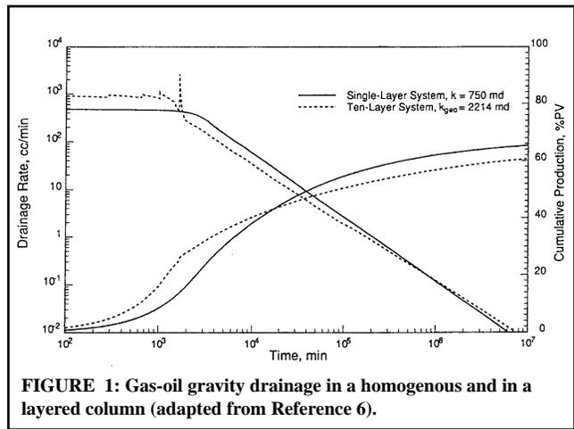
FIGURE 1: Gas-oil gravity drainage in a homogenous and in a layered column (adapted from Reference 6).
