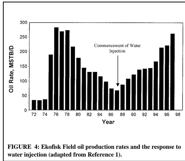
FIGURE 4: Ekofisk Field oil production rates and the response to water injection (adapted from Reference 1).
