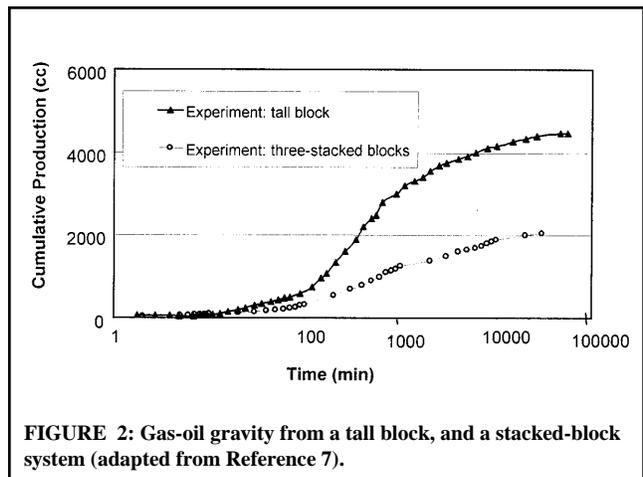
FIGURE 2: Gas-oil gravity from a tall block, and a stacked-block system (adapted from Reference 7).
