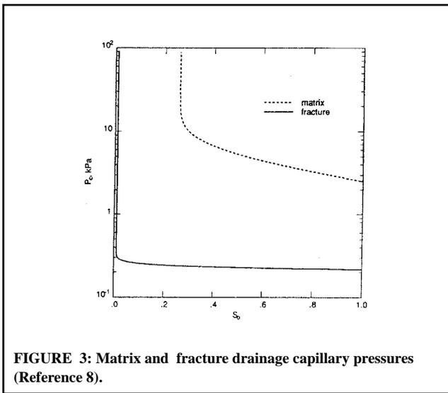
FIGURE 3: Matrix and fracture drainage capillary pressures (Reference 8).
